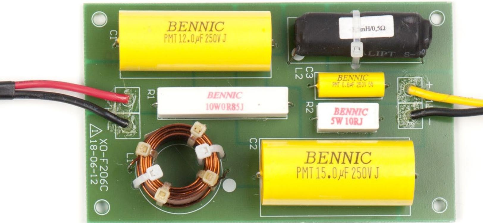
Only the finest materials and internal components have been used for Revel Performa3 loudspeakers, including air-core inductors and audiophile-grade polypropylene capacitors in the crossover network, and heavy-duty gold-plated binding posts. Depending on the model, a tweeter level control allows the speakers' high-frequency balance to be fine-tuned, and a Boundary control enables the speakers to be tailored to individual room acoustics and placement positions.
